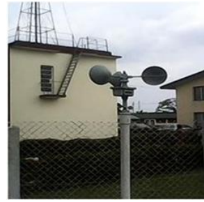
Fig. 3. Anemometer (Wind Speed)
